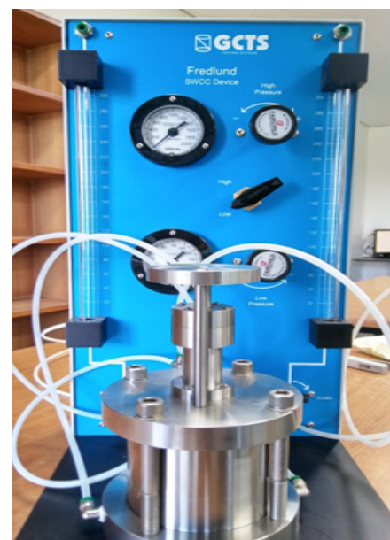
Fig. 2. Experimental setup for soil-water characteristic curve test
