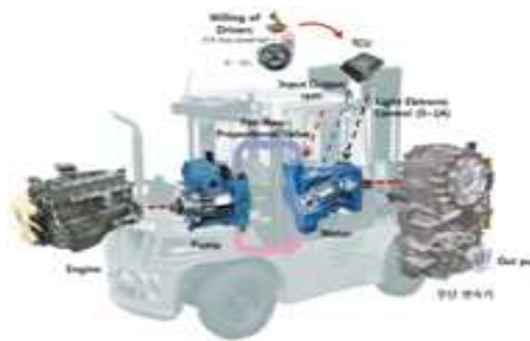
Figure 1. Schematic structure of HMCVT for 8 ton class forklift
