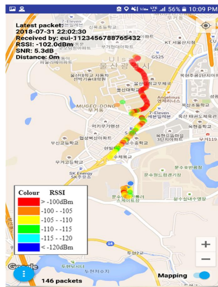
Figure 8. RSSI of received packets at the gateway located at the Kirin House at the University of Ulsan as the sensing nodes moves from the gateway.
