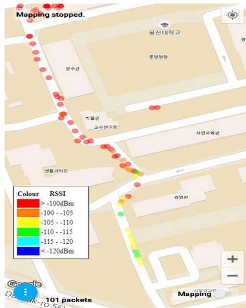
Figure 6. RSSI of received packets at the gateway located at the 6th floor of Department of Electrical and Electronic Engineering at the University of Ulsan as the sensing node moves from the gateway.
