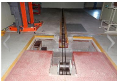
Fig. 2. Rear impact simulator
