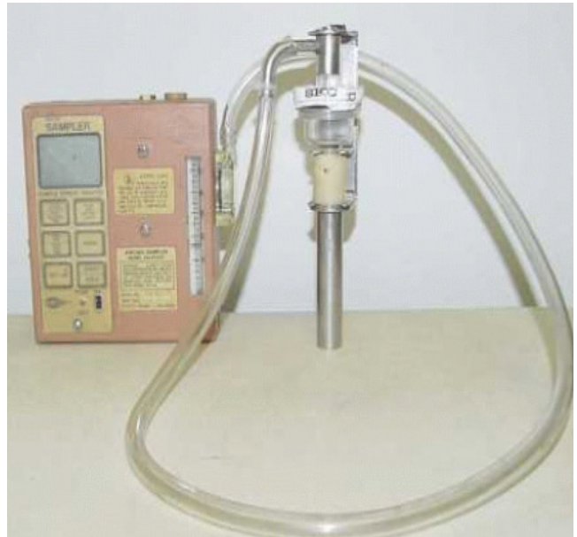
Fig. 1. A sampling cassette and a Dorr-Oliver sampling head for DPM measurements.
