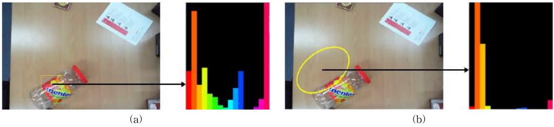
Fig. 4. Result about CAMshift and its color histogram (a) query ROI and (b) conventional CAMShift.
