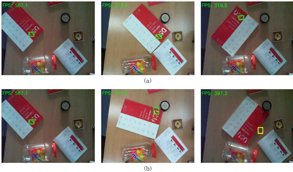
Fig. 11. Experimental result about object tracking with changing illumination condition. (a) result about proposed method (b) result about conventional CAMShift.
