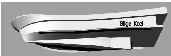
Fig. 2. Bilge keel attached to fishing vessels.
