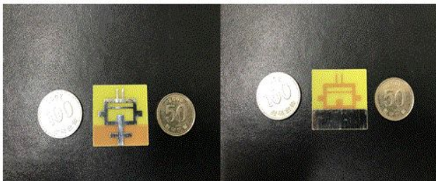
Fig. 11. The front and back of the manufactured antenna.
