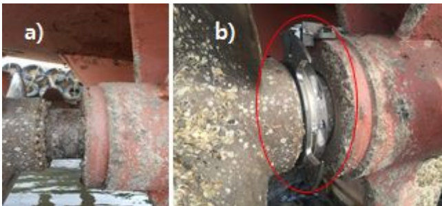
Fig. 1. Propeller shaft of test ship a) before installing, b) after installing rope cutter (F4).
