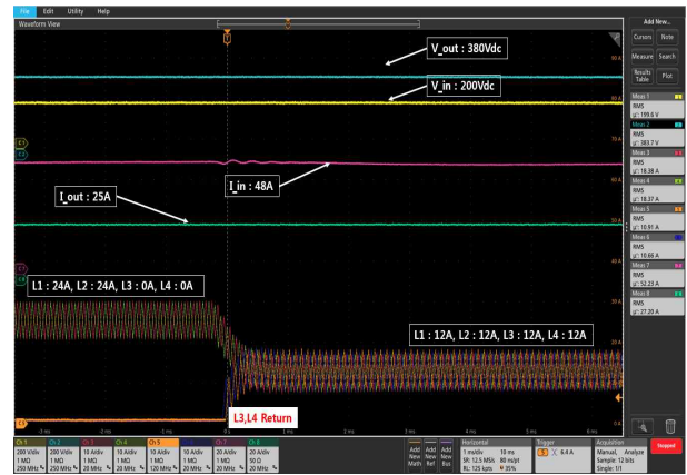
(b) Response wave form of fault return in discharge mode
