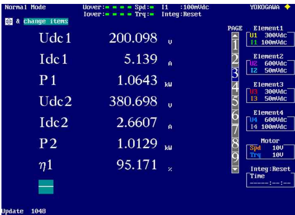
(a) Efficiency data with 10% load
