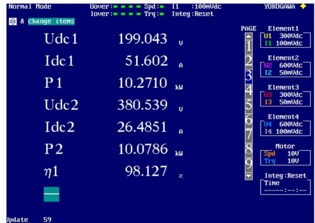
(b) Efficiency data with 100% load
