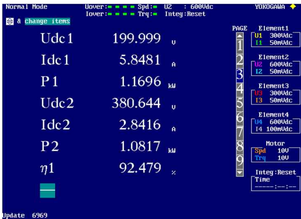
(a) Efficiency data with 10% load
