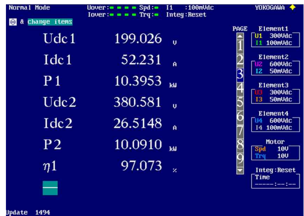
(b) Efficiency data with 100% load
