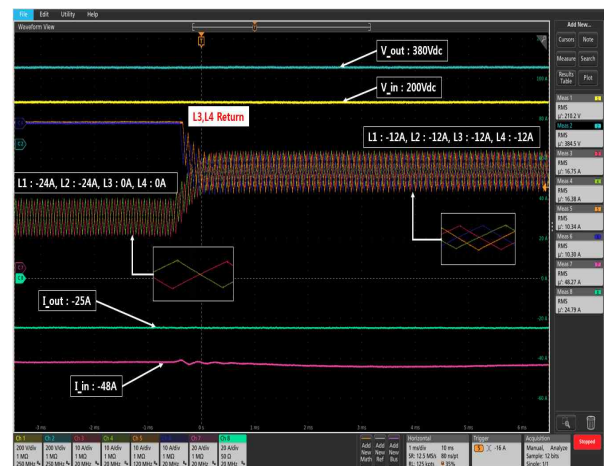
(b) Response wave form of fault return in charge mode
