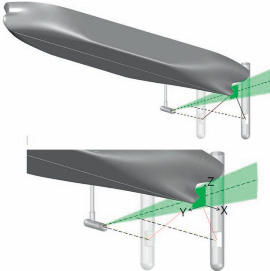
Fig. 2. A schematic drawing of the SPIV setup for wake measurements.
