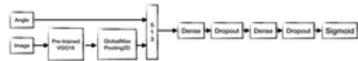
(Figure 9) The same final model as Figure 6. It is compressed into 512 one-dimensional information by Global MaxPooling2D, and is connected to angle information, and 513 are input to a fully-connected layer.
