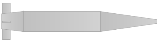
Fig. 2. Configuration of the guided munition as an input to Missile DATCOM
