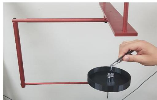
Fig. 7. Configuration of the repeatability experiment by using weights of classes M1
