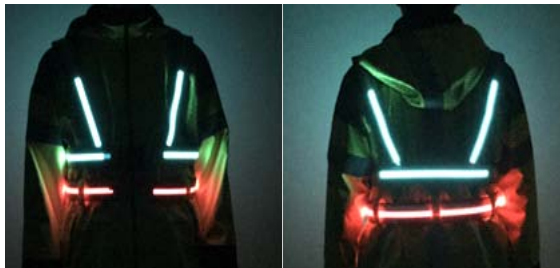
<Fig. 19> Luminous vest & belt prototype using EL tape. Photographed by the author. (March 14, 2017).
