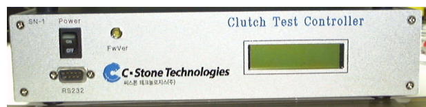
Fig. 4 Embedded controller for clutch test
