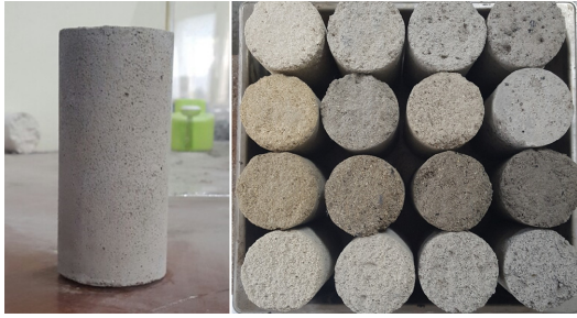
Fig. 1. Concrete test pieces prepared for this study.
