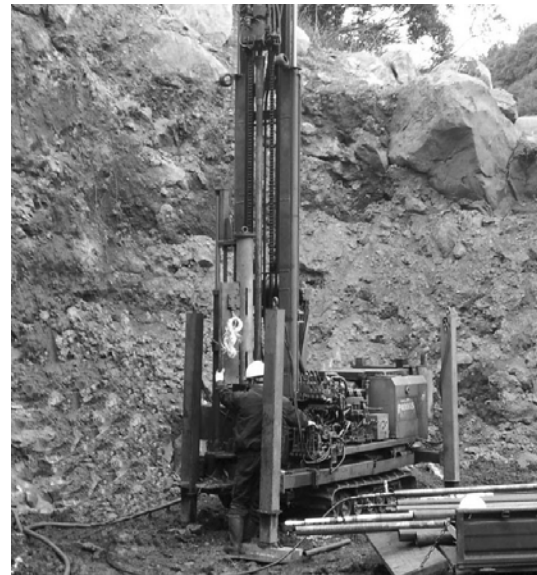
Fig. 2. Hydraulic type drilling machine used in this study.
