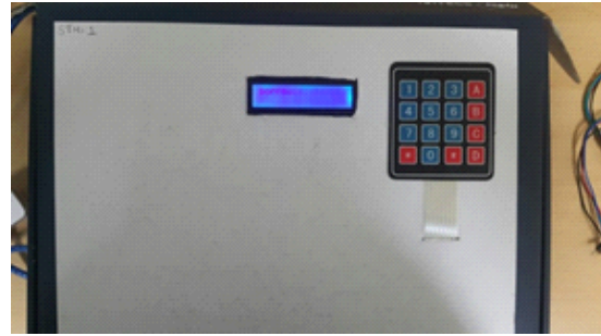
Fig. 4 Control box with a 2x16 LCD and a keypad
