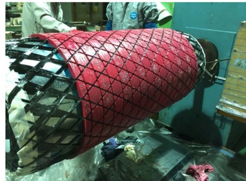
Fig. 2. Fiber winding process of composite lattice structure
