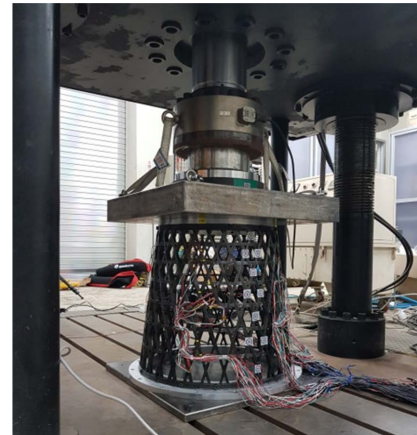
Fig. 9. Compressive Test of cone-type composite lattice structure
