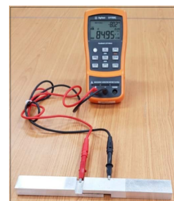
Fig. 6. Measurement of electric resistance by LCR meter
