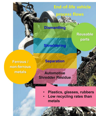
Fig. 1. Recycling process of disused cars
