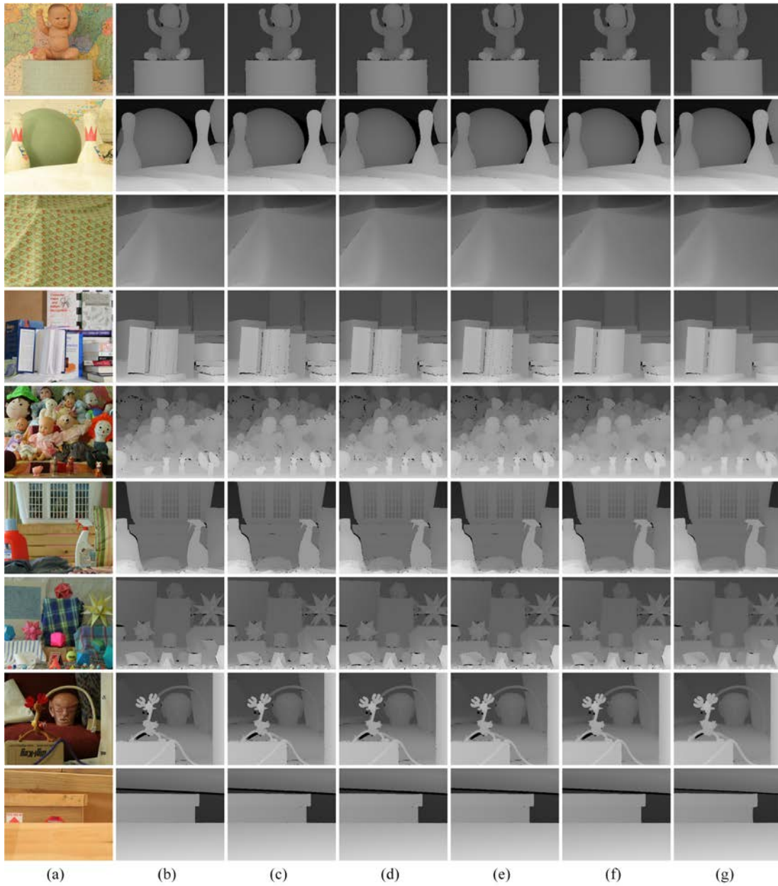
Fig. 4. Results of Baby , Books , Bowling , Cloth , Dolls , Laundry , Moebius , Reindeer and Wood . Down-sampling factor is 4. (a) high resolution color image, (b) ground truth high resolution depth image, (c) results of BI, (d) results of JBU, (e) results of FEDIU, (f) results of DADU and (g) results of the proposed method.
