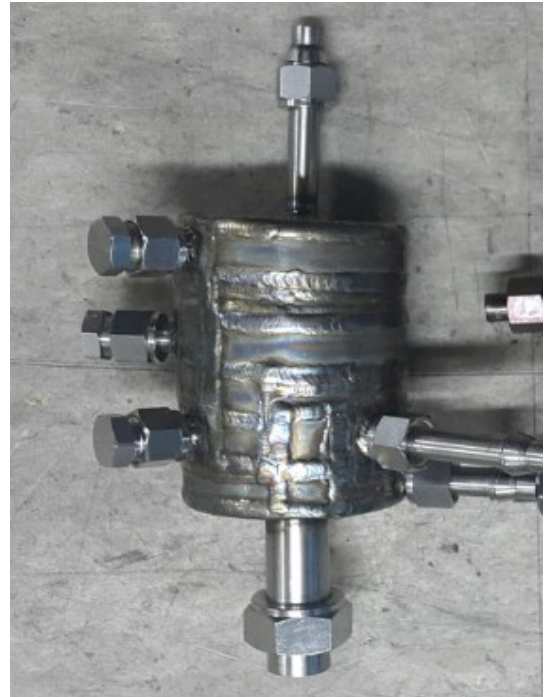
Fig. 3. Photo of reforming reactor
