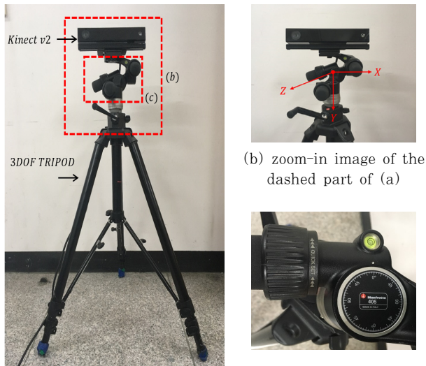
Fig. 7 Experimental set-up of 3D scanning
