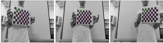
Fig. 4 Intrinsic parameters experiment using checkerboard
