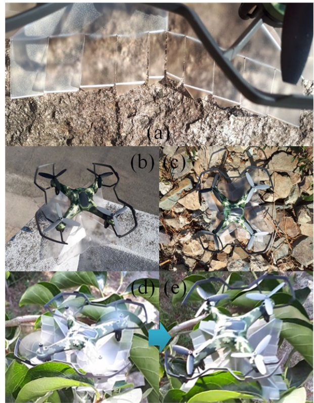
[Fig. 11] Perching test on the different surfaces. (a) Compliant spine on the rock and quadrotor with perching mechanism on (b) the rooftop and (c) a gravelly field. (d) Landing and (e) perching process on the tree bank.
