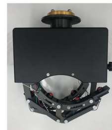
[Fig. 6] Tourniquet gadget: tourniquet gadget control module and 2 jaws with air cuff
