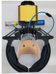
[Fig. 4] Oxygenation gadget: oxygenation gadget control module, 2-jaws with air cuff, and cervical collar
