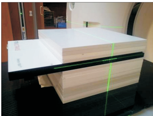
Fig. 2. Patient-specific QA phantom including fiducial-inserted solid water phantom and Octavius 1000SRS detector.
