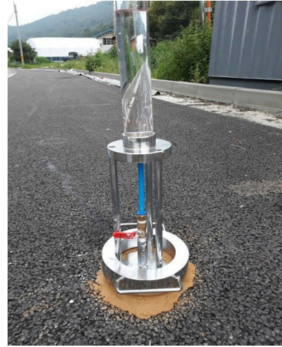
Fig. 11 Pavement Permeability Test Equipment
