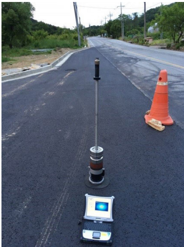
Fig. 10 LFWD Test Machine
