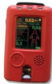
Fig. 1. PED was used to measure occupational radiation dose manufactured by Tracerco™.
