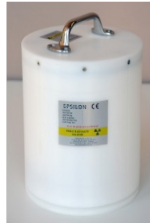
Fig. 3. 68 Ge cylinder phantom was used for measuring uniformity of PET imaging according to the Standard Operation Procedure of Quality Control.
