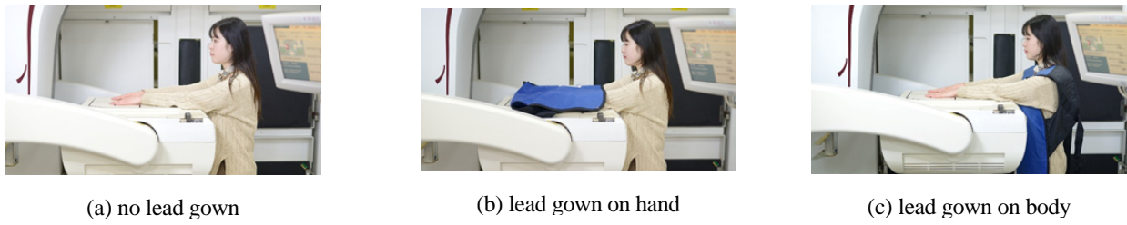
Fig. 6. A lead gown was used to remove scatter ray from body (a)–(c).
