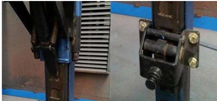
Fig. 3. Upper stop device for pneumatic cylinder and lower stop device for return.
