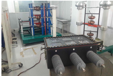
Fig. 5. Photograph of 3 Stage, 300 kV LI Generator connected to the 22 kV circuit breaker specimen
