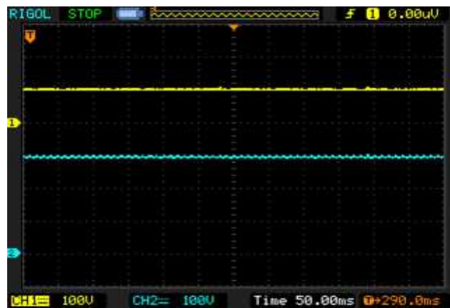
Fig. 16. Voltage across the individual capacitor (CH1) and Total voltage across the capacitor (CH2) for D=0.5
