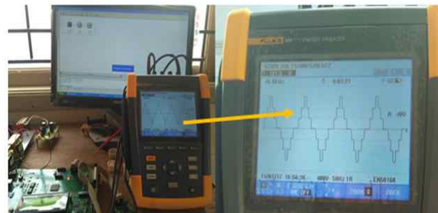
Fig. 15. 1- \phi seven-level BDCLCRV MLI output voltage for R-Load
