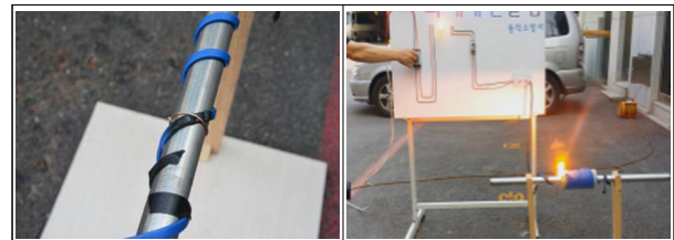
Fig. 16. Fixed by copper wire to damaged positive temperature wire, burn the thermos with spark.
