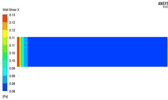
Fig. 14. Wall shear stress contour at pipe wall
