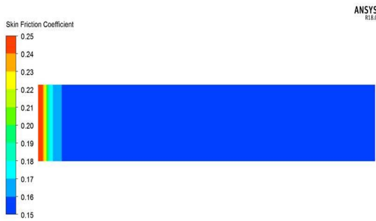
Fig. 15. Skin friction coefficient contour at pipe wall
