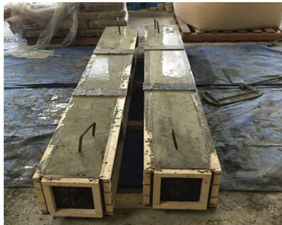
(c) Finishing of slurry filling
