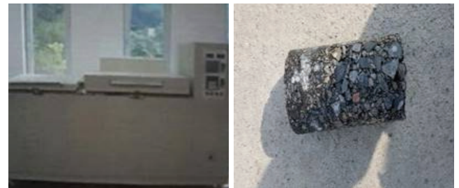
Fig. 15 Freeze-thaw tester and specimen
