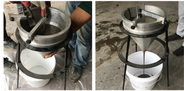
Fig. 2 Flow test of cement grout
