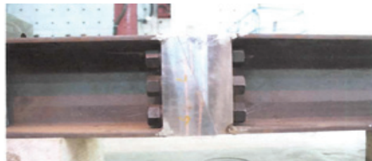
Photo 7 New modular junction test specimen
