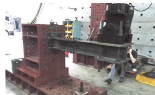
Photo 11 Installation condition of existing joints
