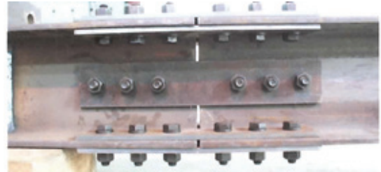
Photo 9 Details of existing joint specimen
