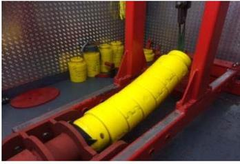
Fig. 11 Bend restrictor test (Supergrip, 2018)
