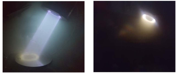
Figure 3. Ion beam shapes generated from an anode type ion beam source; (a) a normal beam shape, (b) an abnormal beam shape.
