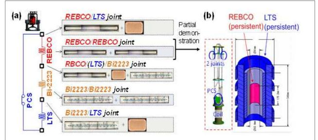
**Figure. 2.** (a) Schematic of an example coil circuit in a 1.3 GHz NMR magnet (option-A in Figure 1). (b) A persistent current 400 MHz (9.39 T) LTS/REBCO NMR magnet with a primitive REBCO inner coil.
