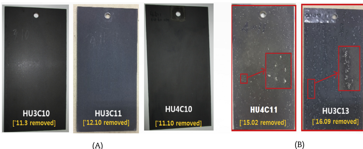
Fig. 1. METAMIC surveillance coupons. (A) Coupons without white spots. (B) Coupons with white spots.
