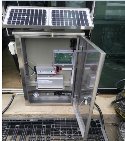
Fig. 2. Outdoor Gateway Control Unit
