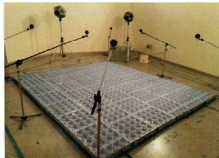
Fig. 2. Photograph of experimental setup of the reverberation room method.
