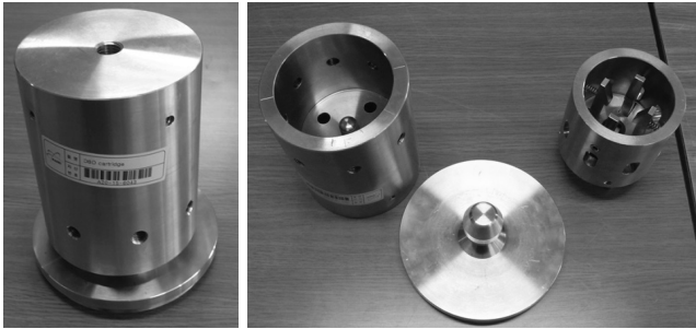
Fig. 3. Compartments (joint body, hook box, and hook) and the assembly of the novel joint device.
