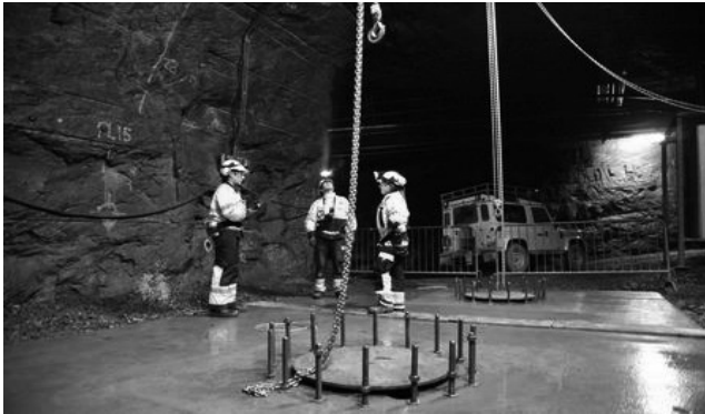
Fig. 10. Testing of Buffer Material at the ONKALO UCRF.
