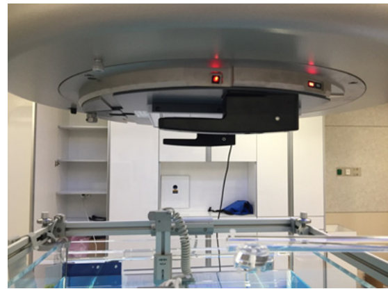
Fig. 1 Setup of stealth chamber mounted on head of LINAC and stealth chamber
